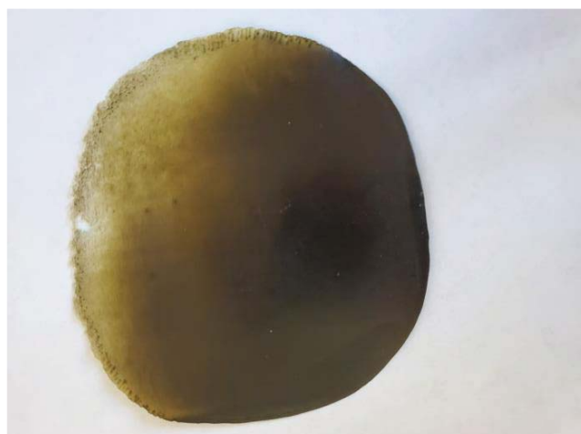
Figure 6 Bioplastic sample containing 30% algae biomass derived from commercially available sources (AA30).
