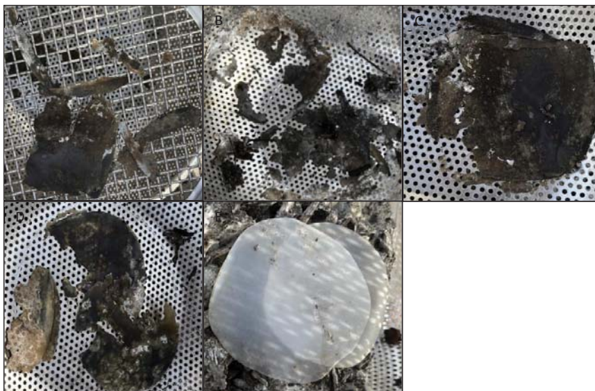
Figure 11 Plastic samples after the first eight-week compost period: AB30 (A), AB30E (B), AA30 (C), BPE0 (D), PE (E).
