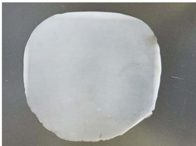
Figure 7 Bioplastic sample containing 0% algae (BPE0).
