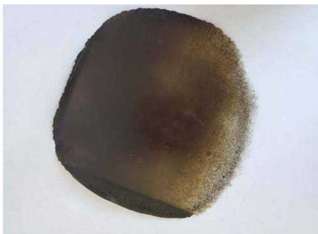
Figure 5 Bioplastic sample containing 30% RABR algae with a biodegradation-enhancing resin (AB30E).
