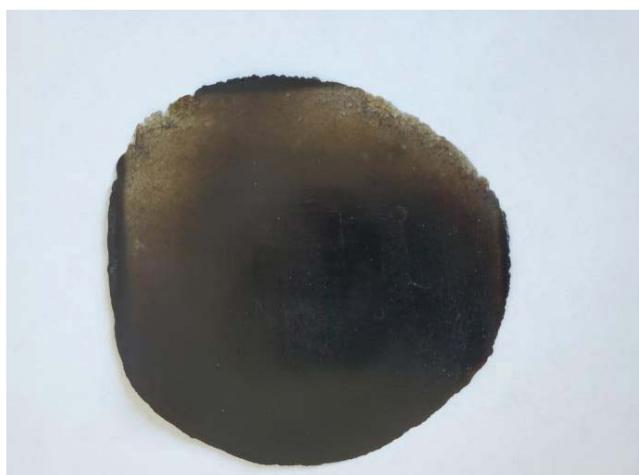
Figure 4 Bioplastic sample containing 30% RABR algae biomass (AB30).
