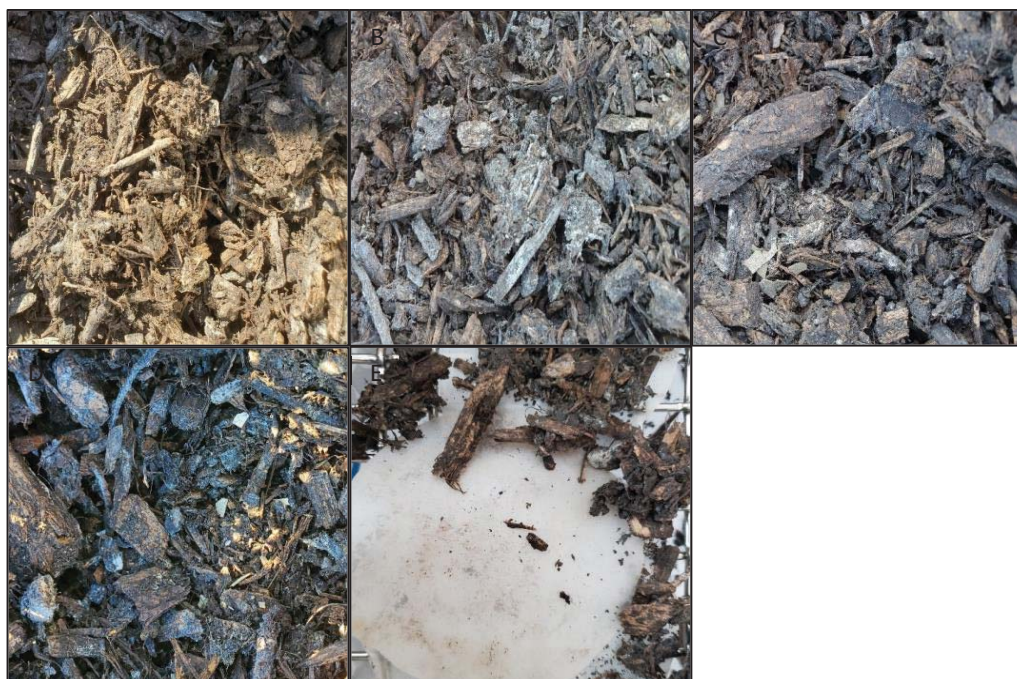
Figure 12 Plastic samples after the second eight-week compost period: AB30 (A), AB30E (B), AA30 (C), BPE0 (D), PE (E).
