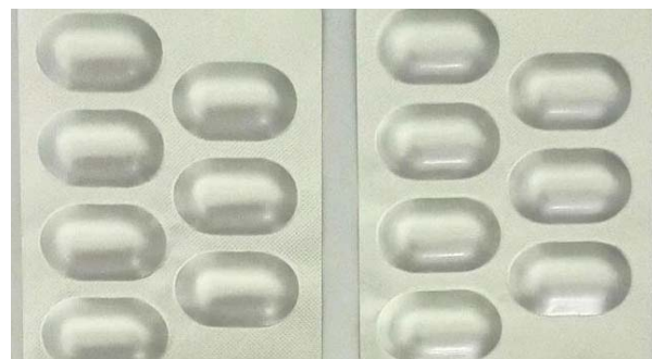
Figure 5 The finished pharmaceutical product of lymecycline (408 mg hard gelatin capsules) was packaged in alu-alu foil to ensure protection from moisture, light, and environmental factors.
