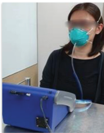
Figure 3 Quantitative Fit Test (QNFT) method using the PortaCount® system.
