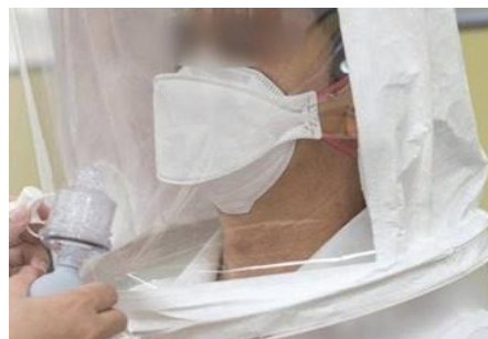
Figure 2 Qualitative Fit Testing (QLFT) using the Bitrex® solution.
