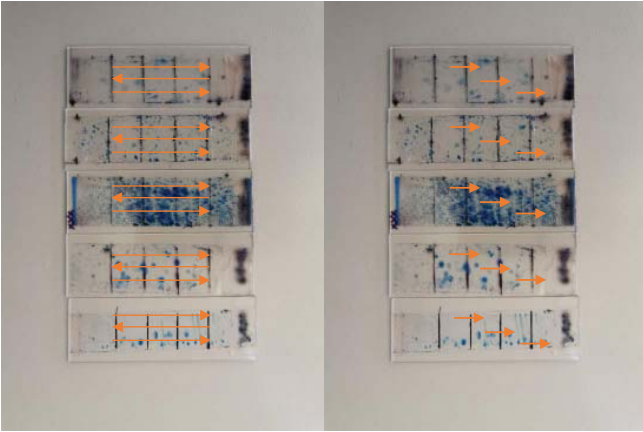
Figure 3 Counting of the adhesive films by the test counters 3 lines and in 3 stages.
